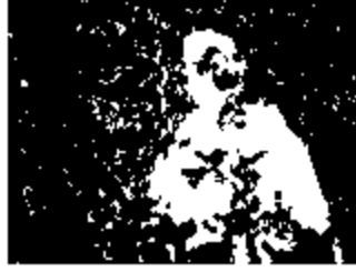
Figure 4.12: Frame differencing result for threshold of 50
