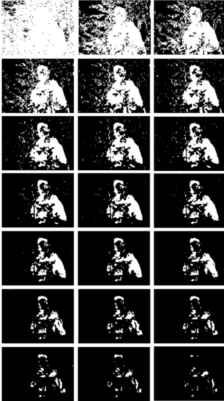
Figure 3.13: Frame differencing with median filtering. Results are for threshold being varied from 0-200
