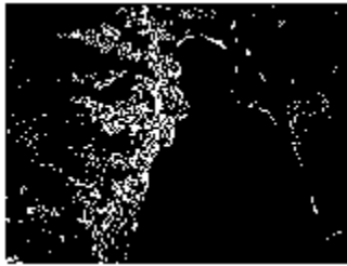
Figure 4.15: Incorrectly detected foreground pixels in the frame differencing result
