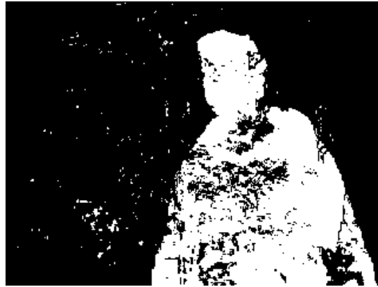
Figure 4.11: Mixture of Gaussians result for the Wallflower data set waving trees challenge
