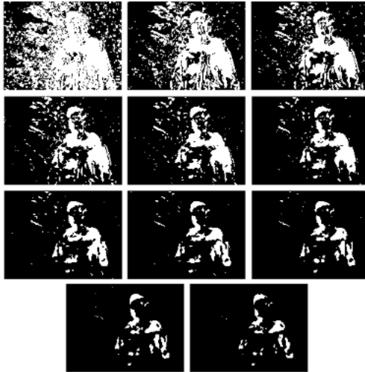
Figure 3.5: Result for approximate median with the threshold varied from 0-200
