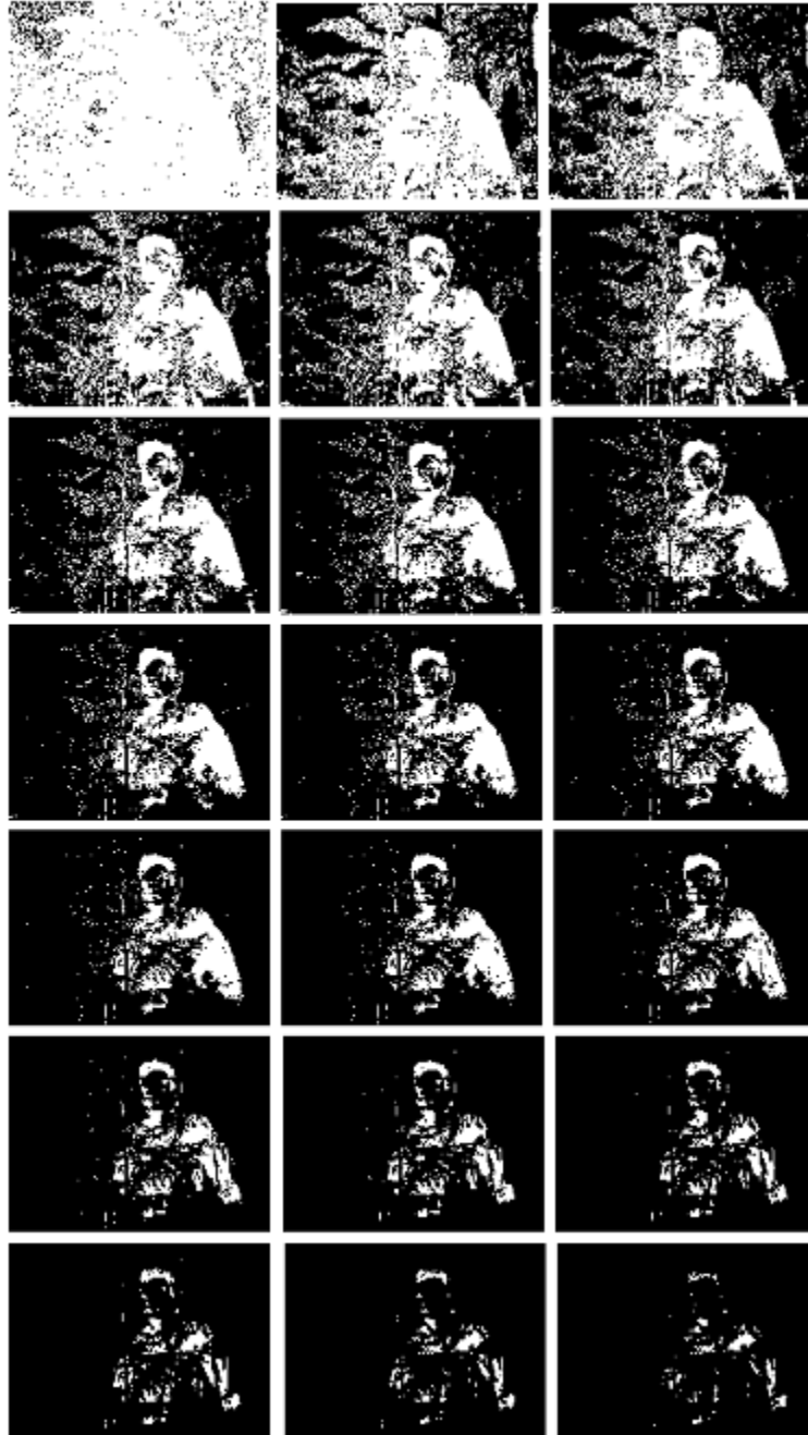
Figure 3.1: Result for frame differencing with the threshold varied from 0-200
