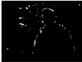
Figure 4.16: Incorrectly detected foreground pixels in the approximate median result
